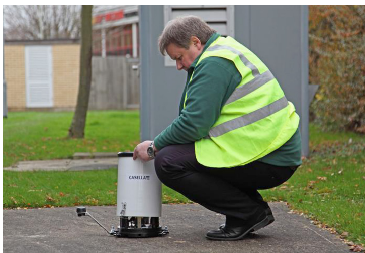
A ‘Storm Guardian’ rain gauge being installed (image courtesy Casella Solutions)
